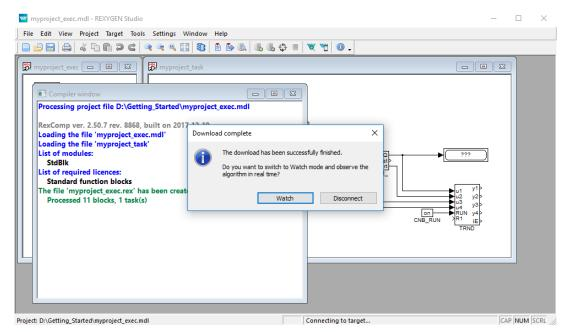
In the *Watch mode*, the background of all files goes gray and you cannot move or delete any blocks or connections. Right-click the TIMER\_ block and select *Watch selection* in the menu to watch the inputs and outputs of the timer.
