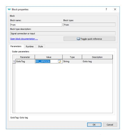
The second physical switch will be connected to GPIO#24 (RPI\_\_GPIO24U).
