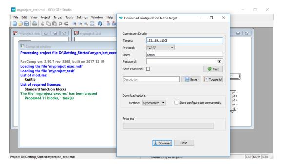
Enter the IP address of your Raspberry Pi in the Target field.
