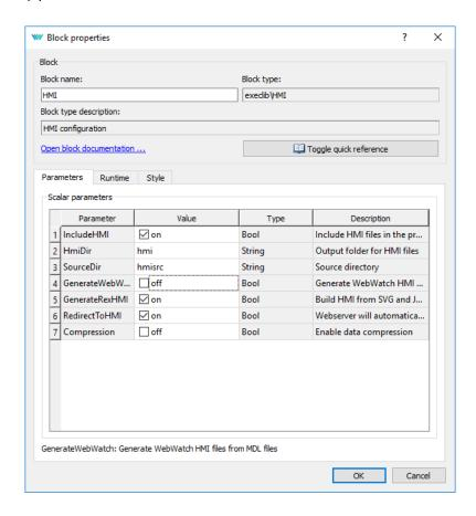
4. The HMI is now an integral part of your project. Compile the project again and you will see that the compile log contains more information. The index.html file is generated from the source index.hmi.js file. All the HMI files are generated into the hmi subfolder (HTML, JS and CSS files) and included in the resulting binary myproject\_exec.rex file.
