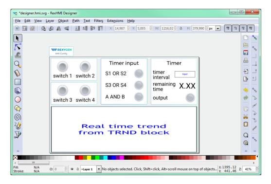
As mentioned earlier, the \*.hmi.svg files in the hmisrc folder are automatically processed while the project is compiled in the REXYGEN Studio application. The project main file must contain the HMI block with GenerateRexHMI parameter enabled. This was already covered in Section 4.3 so you should have everything ready.
