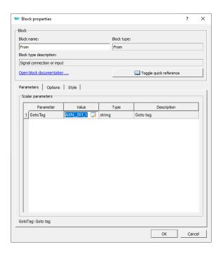
The other physical switch (SW3) is connected to Digital Input 1.3 (AXN\_\_DI1\_3). The last (Digital Output) flag will be set as GotoTag = AXN\_\_DO1\_1
