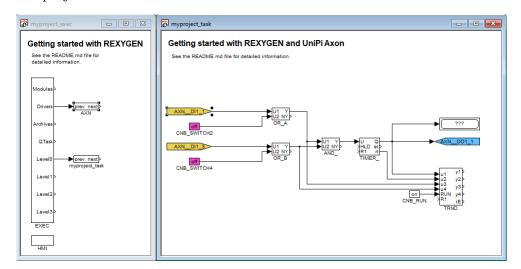
After compiling the project and downloading it to the UniPi Patron the control algorithm interacts with the physical world. Again it is possible to switch to Watch mode and observe the signals in real-time or analyze the trends of signals. Flip the physical switches and watch the signals.
