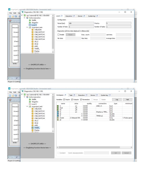
Now you can switch REXYGEN Studio back to the *Development mode*. You can do so by deactivating the *Watch mode* (use the  $\blacksquare$  icon). You are offered synchronization of the changed parameters with the source files of the project, choose No at this moment.
