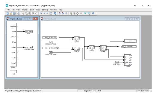
After compiling the project and downloading it to the WAGO PFC100/200 the control algorithm interacts with the physical world. Again it is possible to switch to Watch mode and observe the signals in real-time or analyze the trends of signals. Flip the physical switches and watch the signals.
