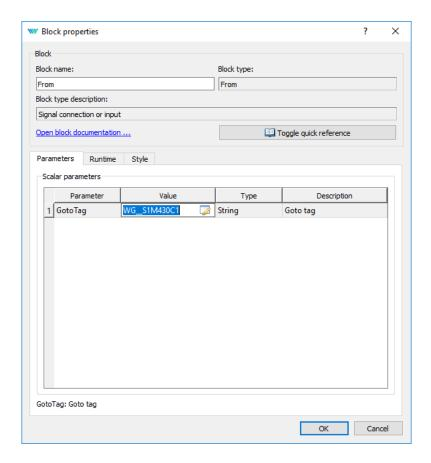
The other physical switch (SW3) is connected to channel 3 of the same module (WG\_\_S1M430C3). Channel 1 of the 750-530 module in memory slot 2 (WG\_\_S2M530C1) will serve as control signal for the external relay.
