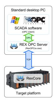
It is necessary to define the IP address of the REXYGEN target device in Windows registry to allow data exchange with the OPC server. Find the following key in the Windows registry
