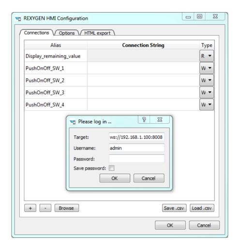
Select *Connection String* field of the <code>Display\_remaining\_value</code> item and afterwards browse the tree to the <code>TIMER\_</code> block and <code>double-click</code> the <code>rt</code> parameter. The connection string of the parameter is copied to the <code>Display\_remaining\_value</code> alias, which is shown in the next figure.
