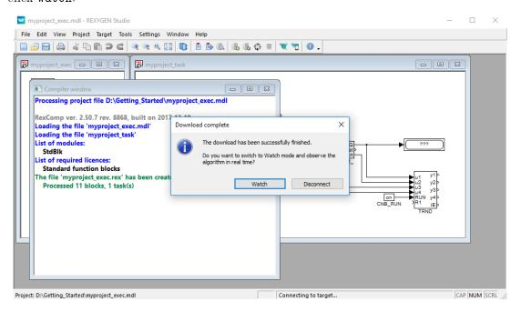
In the *Watch mode*, the background of all files goes gray and you cannot move or delete any blocks or connections. Right-click the TIMER\_ block and select *Watch selection* in the menu to watch the inputs and outputs of the timer.
