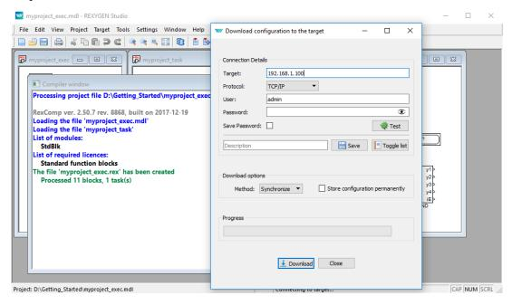
Enter the IP address of your platform in the Target field <sup>2</sup>.
