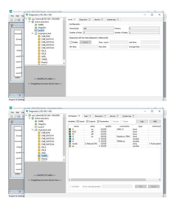
Now you can switch REXYGEN Studio back to the *Development mode*. You can do so by deactivating the *Watch mode* (use the icon). You are offered synchronization of the changed parameters with the source files of the project, choose No at this moment.
