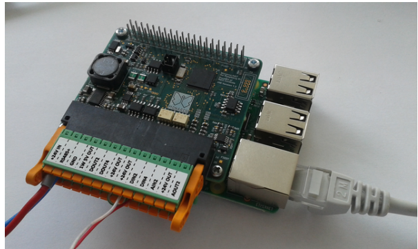
Figure 3.2: Terminal pinout for Monarco HAT.
