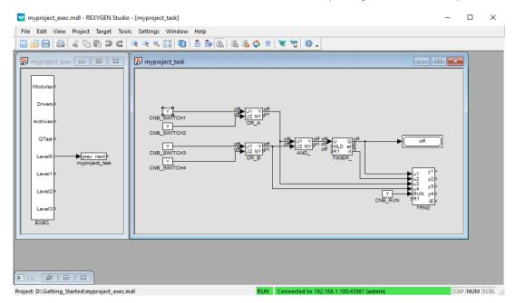
Now it is possible to double-click the CNB\_SWITCH1 block and change the Boolean variable to YCN = on (tick the checkbox and click OK). Once you do the same with the CNB\_SWITCH3 block, the outputs of both OR blocks are on and the Y output of the AND\_ block goes on and the TIMER\_ starts to count down. Observe the rt output.<sup>3</sup> Once the
