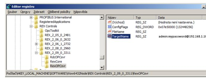
Afterwards it is possible to establish data exchange with the running executive of the REXYGEN system from the visualization software. The OPC server named REXControls.RexOPCsvr allows the visualization SW to read all inputs, outputs and parameters of the function blocks the control algorithm is composed of. It is possible to write to function block parameters and inputs. For the latter case, no signal can be connected to the block input in the control algorithm.
