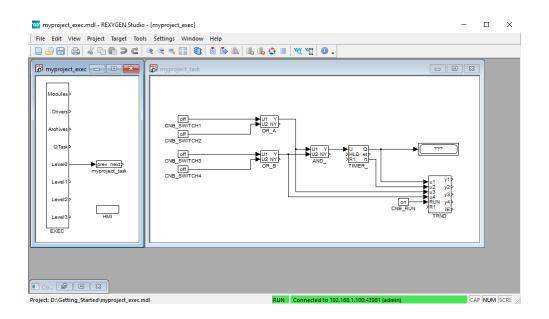
3. Double-click the HMI block to edit its parameters. Set GenerateWebWatch = off and confirm. WebWatch is another type of HMI, which you do not need at the moment. See [4] for details, it is a very interesting tool for developers and technicians.
