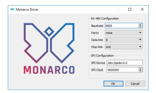
As the final step, rename the IODRV block to MNR, which will serve as a prefix for all I/O signals of this driver.
