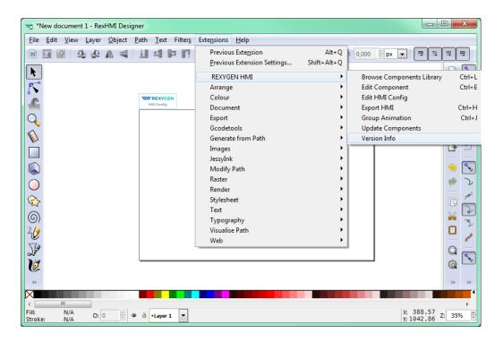
This extension adds a special component which contains general settings of the HMI. Close it with the OK button for now.
