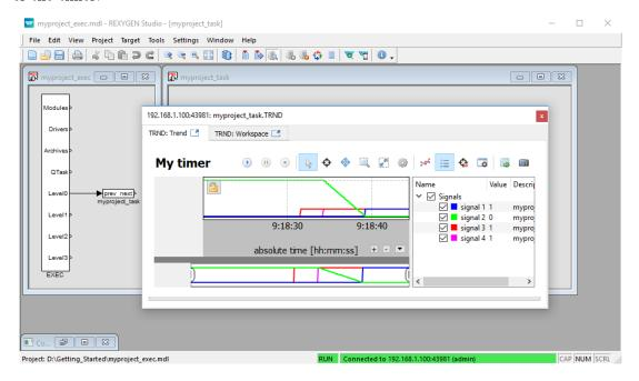
Try turning the CNB blocks off and change the pt parameter of the TIMER\_ block. Afterwards turn the CNB blocks on again and observe the signals in the TRND block again. As you can see, you can modify any parameter in real-time, which allows you to fine tune your algorithm.
